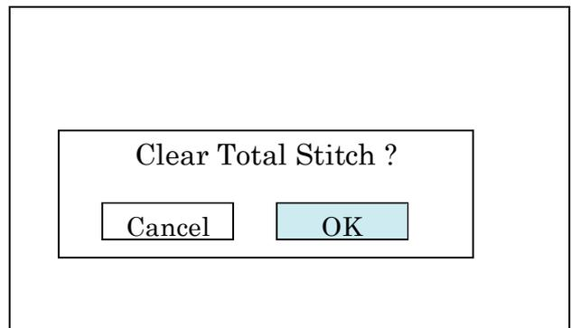
\* Total number of stitch is cleared after pressing **OK** and the screen shows one in the procedure 3. Total number of stitch is 0.
