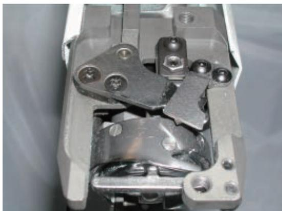
7. On Checking that the knife began to open, at [116 degrees (+0 / -2degrees)] work has finished.
