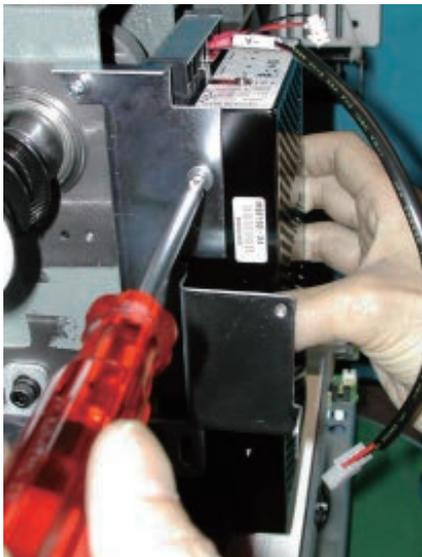
2. Loosen screw on thread cut cam.
