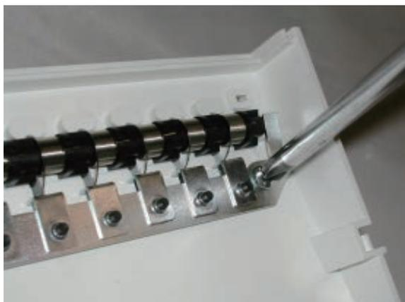
3. Remove thread adjusting spring ass'y.
