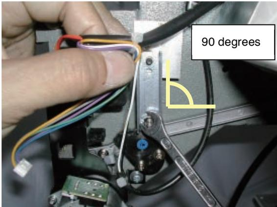
12. Adjust the height of pressure foot guide bar.
