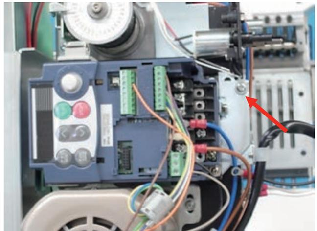
4. Tighten screws with screwdriver to install power cable and motor cable per the following connection diagram.
