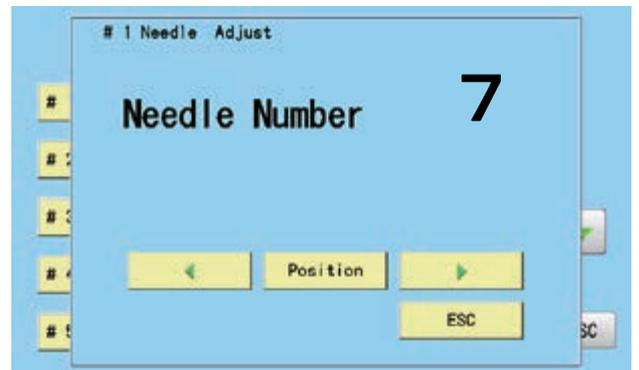
5. Turn knob so that the needle position can be the 6<sup>th</sup> needle.
