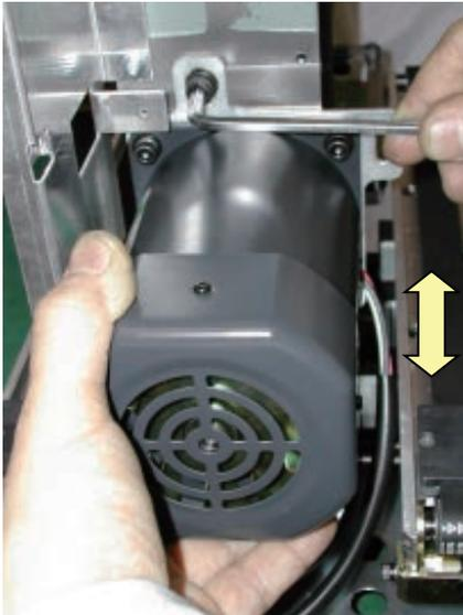
5. Tighten screw on motor bracket.
