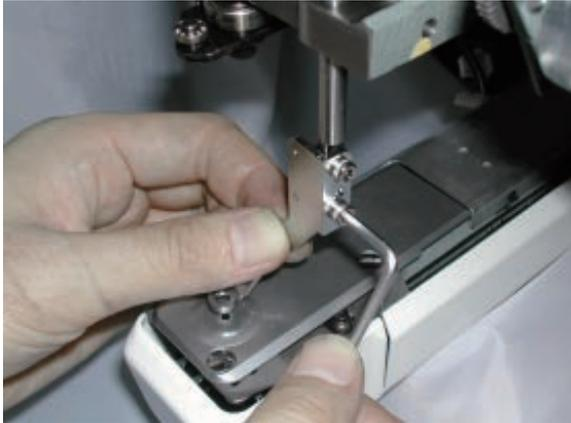
7. Adjust the height of pressure foot guide bar to finish.
