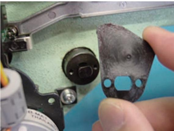
3. Put on grease to pressure foot cam.
