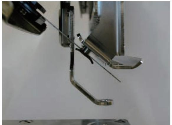
5. Thread catcher device should be adjusted if above clearance is not keepable.
