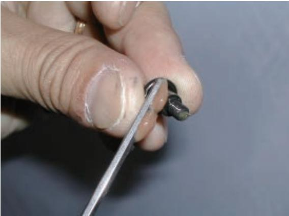
8. Assemble pressure foot drive lever ass'y.
