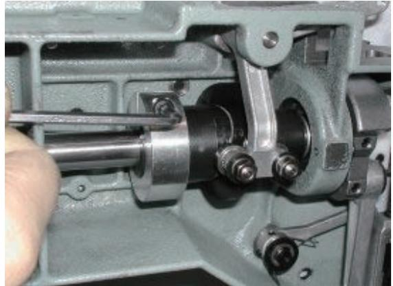
5. Loosen screw on crank.
