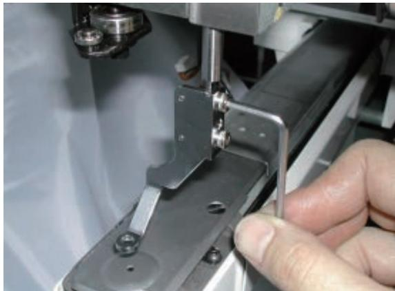
2. Loosen the screw which fixes guide bar block.
