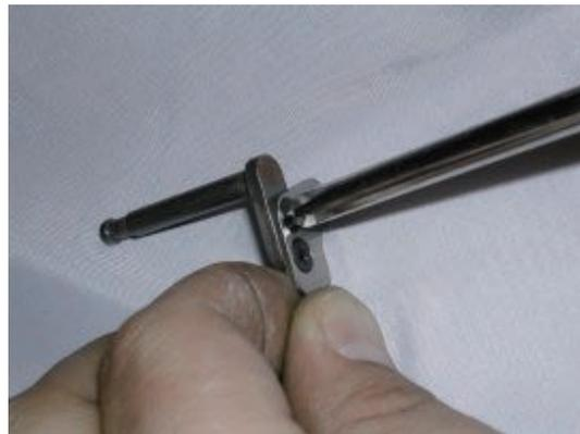
5. Setting drive link hole to moving knife, insert knife drive shaft assembly.
