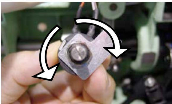
Turning the shaft too much make \* disappear, and turn the shaft back and forth, and adjust the position so that continuous beep is made.
