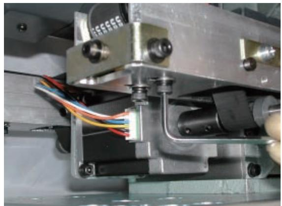
9. Tighten lock nut for tension adjustment screw.
