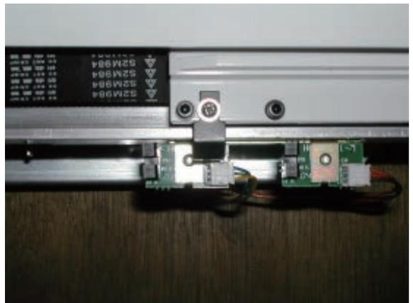
7. Adjust by bending detecting plate by hand if you find any interference with sensor or connector.
