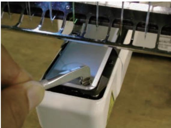
2. Remove knife drive shaft retainer.
