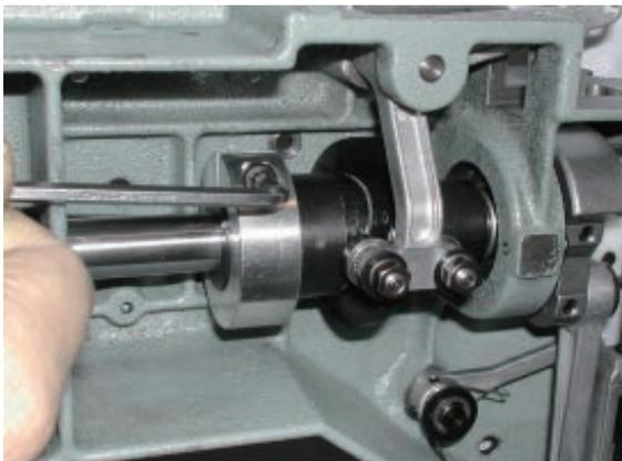
12. Loosen screw on crank.
