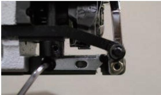
2. Insert keeper positioning gauge (Bobbin) into rotary hook.
