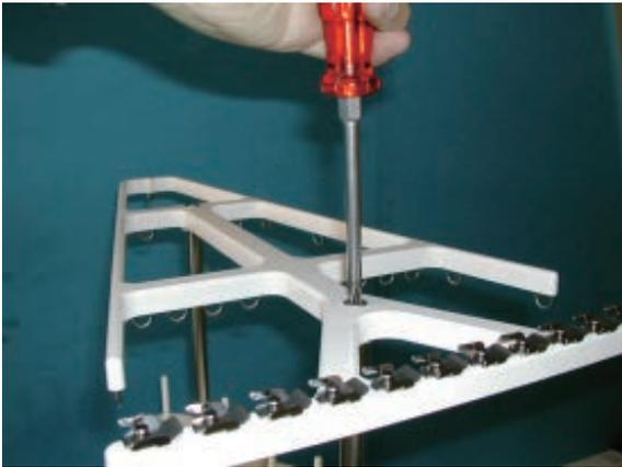
6. Loosen a screw of thread guide pillar
