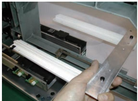
5. Loosen lock nut for tension adjustment screw.
