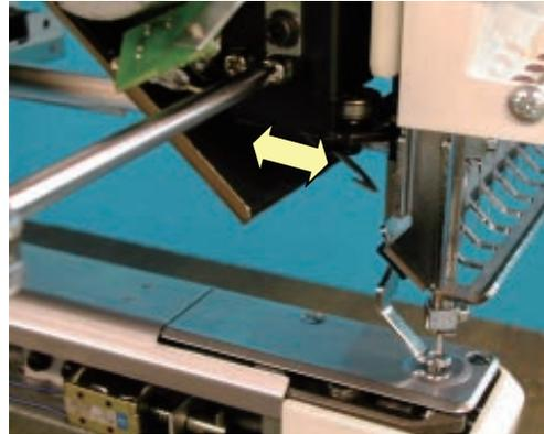
\* Insert Lower rail to between the two bearing deeply.
