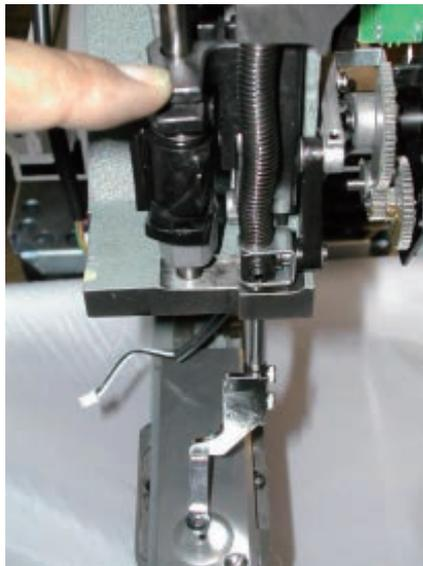
5. Adjust the center between needle hole of needle plate and hole of pressure foot.
