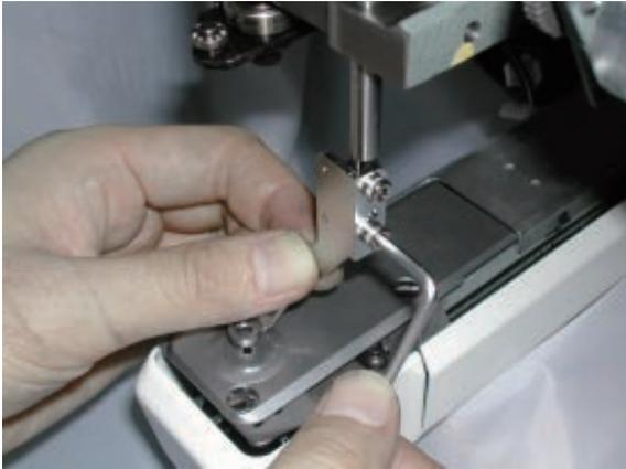
2. Loosen the screw which fixes guide bar boss.
