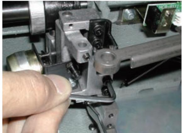
9. Remove thread cutting roller.
