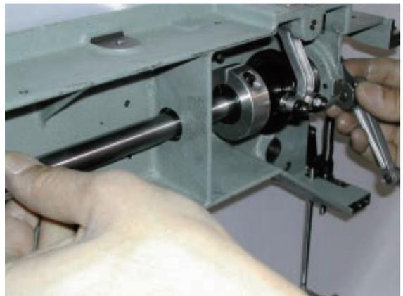
14. Remove bearing retainer.
