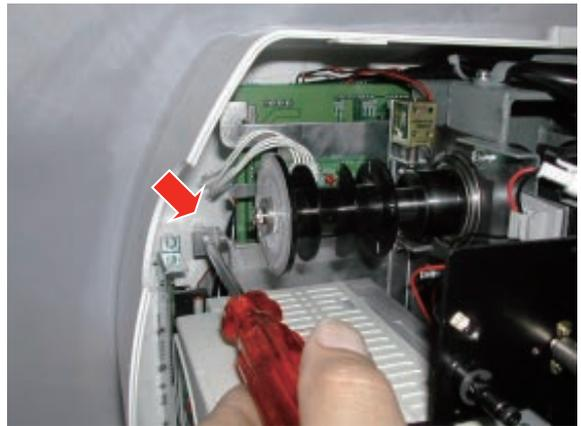
17. Remove an arrow marked screw which fixes hold arm D.
