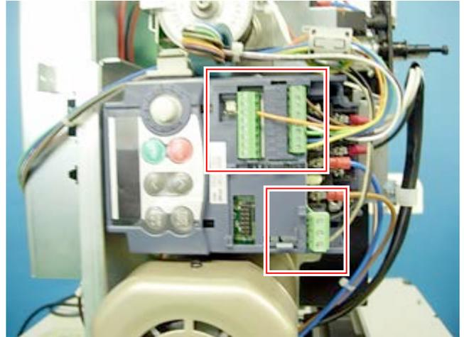
5. Remove screws with Phillips screwdriver and remove power cable and motor cable.
