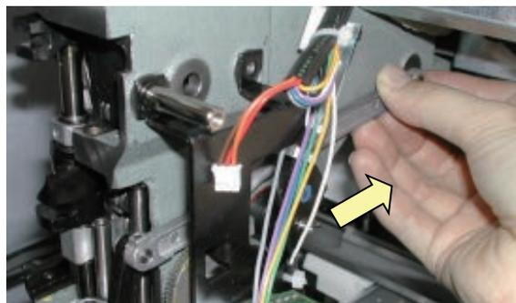
6. Put on grease to body and oil bush of pressure foot lever ass'y.
