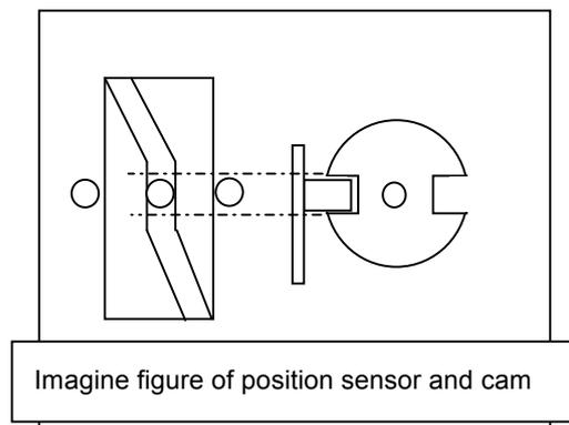
2. Set position where sensor on sensor board and slit don't cross to area where moving head doesn't move when turning groove cam.
