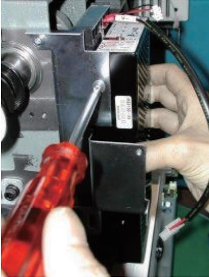
2. Remove timing detecting board ass'y.
