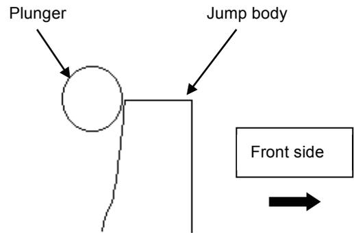
7. Adjust upper shaft to be [180 degrees] and tip of the body has to be same as the picture below.
