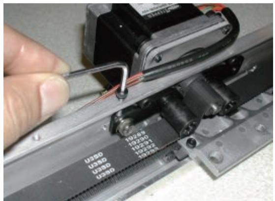
7. Remove the screw which fixes tension bracket.
