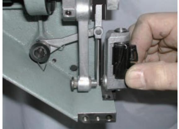
3. Loosen screw on rod pin to remove rod.
