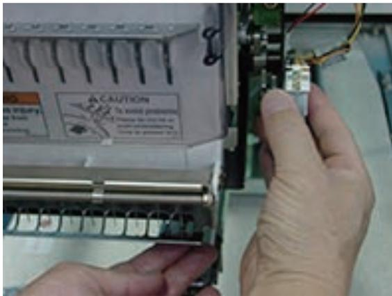
3. Adjust the position of the pressure foot bracket ass'y.
