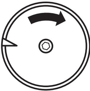
4. Move circuit board up and down and set to position where LED 2 disappears at [0 degree], then fix with screw.
