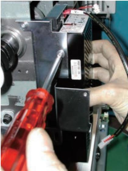
10. Loosen screw on upper shaft collar, upper pulley, drive pulley.
