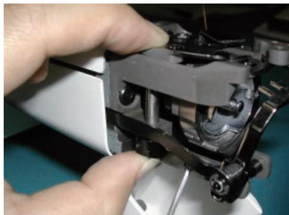
7. Referring to [3-6-8 Adjustment of moving knife and fixed knife], check how well thread is cut and adjust, then finish this process.
