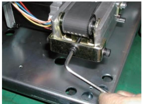
8. Tighten screw on tension.
