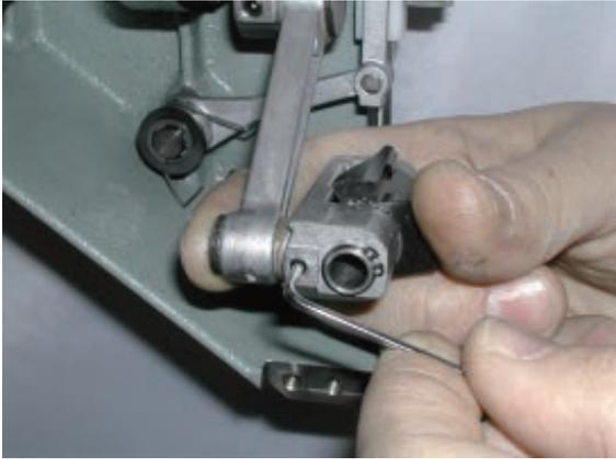
5. Remove needle bar driver ass'y.
