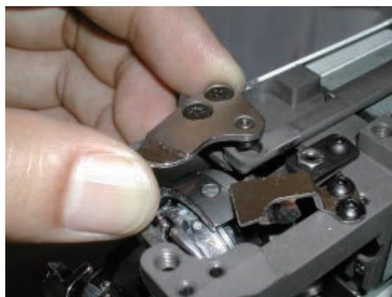
6. Pushing down moving knife and knife drive shaft retainer like putting them together, fix knife drive shaft retainer.
