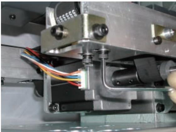
7. Adjust belt tension, to use belt tension gauge.
