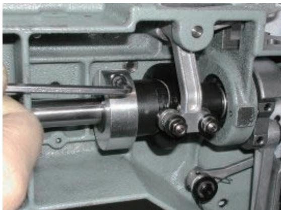
5. Loosen screw on crank.
