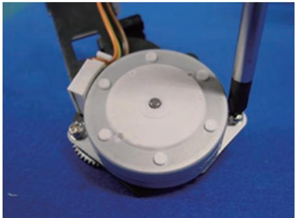
6. Assemble the drive gear A.
