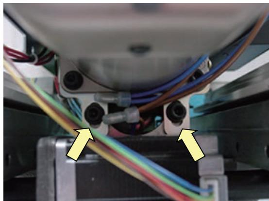
4. Adjust motor belt tension.
