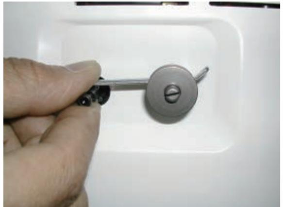
If the guide touches the bobbin adjust position of the winder bracket ass'y.
