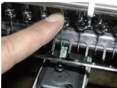
6. Turn an upper axis up to [302 degrees - 303 °], and it is the needle mark to a seal. A hole is made.
