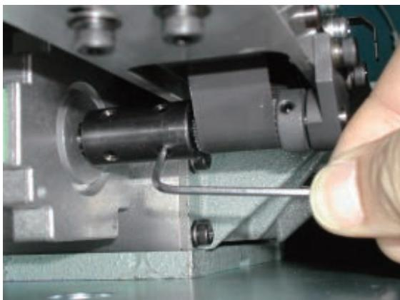
4. Remove the screw of Y carriage bracket (left).
