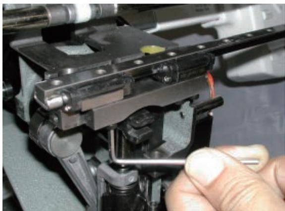
3. Remove pressure foot and pressure foot guide bar.
