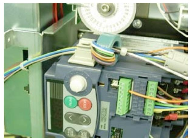
7. Remove two screws shown in the following figure and inverter.
