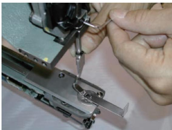
7. Before terminates the adjustment, reconfirm procedure 5, Needle hole of needle plate and hole of pressure foot to be centered.
