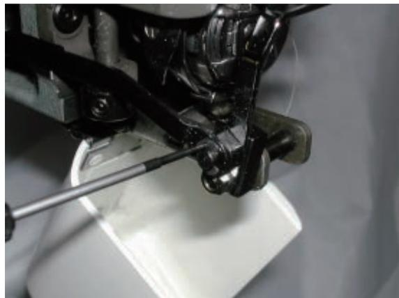
3. Remove keeper solenoid ass'y.
