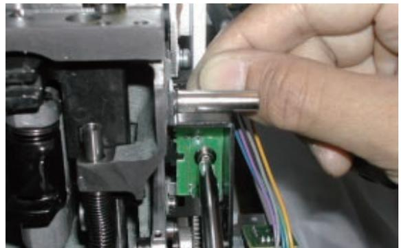
11. Adjust position of pressure foot guide plate A ass'y.
