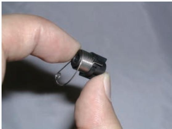
5. Exchange thread adjusting spring.
