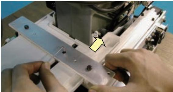
3. Hold the left side of arm to body and tighten screw.
