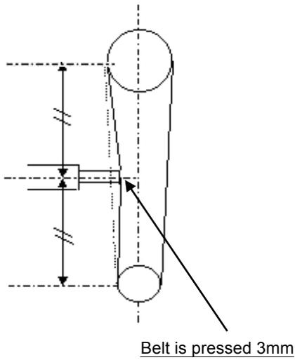
Move main motor upward and downward to adjust.
