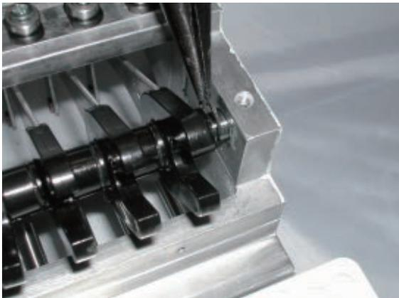
8. Remove the take up lever shaft first then remove the take-up lever.
