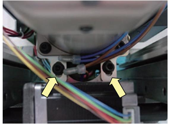
6. Return power supply bracket, power supply, bobbin winder and inverter to previous places to finish.
