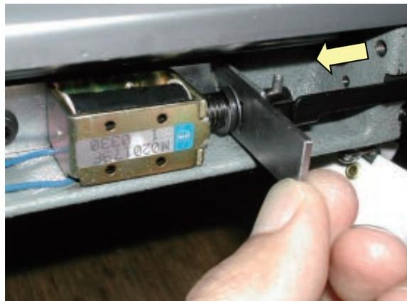
4. Adjust solenoid base where tip of keeper contacts slightly to the gauge then tighten bracket screw.
