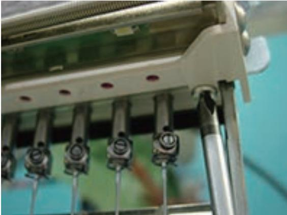
2. Block has spring groove to be able to adjust in three steps
