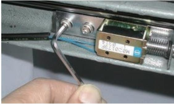
Loosen screw on stopper bracket.
