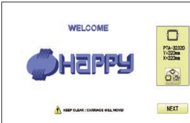
3. Press **NEXT** while pressing **START/STOP** button at the screen of the control box after booting the machine.
