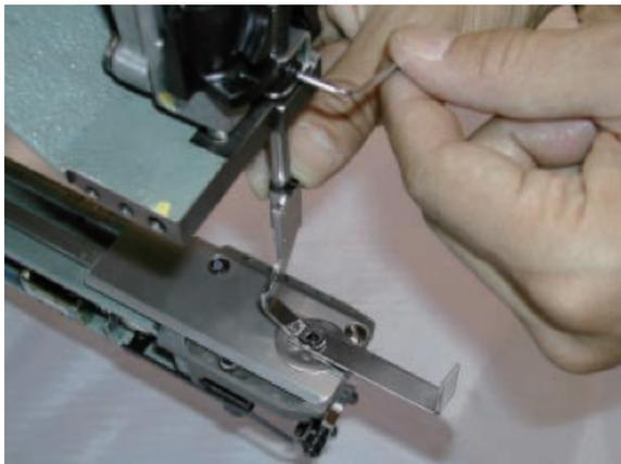
13. Assemble the upper rail of moving head.
