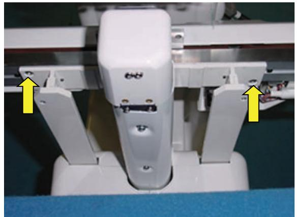
10. Remove the thread tension ass'y.
