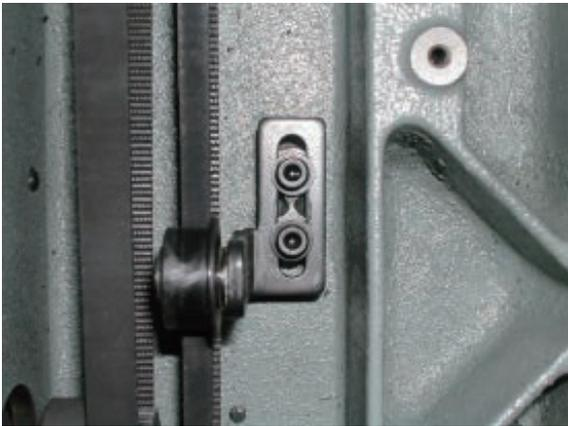
Please move tension shaft ass'y upward and downward to adjust.
