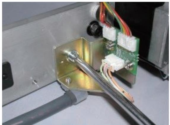
6. Loosen screw for tension.
