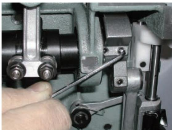
6. Pull out upper shaft (to the extent that shaft comes off from take-up lever cam).
