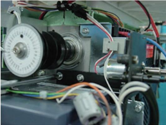
2. Fix 2 screws tentatively timing detecting board.
