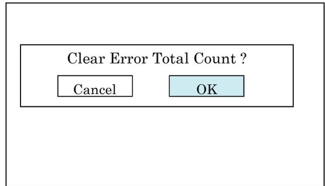
\* Error record is cleared by pressing **OK** and the screen of
