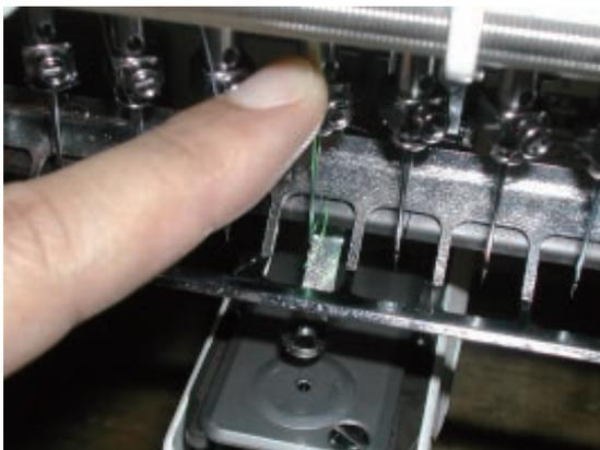
3. Turn upper shaft and set needle near to the lowest needle position [L] to adjust positioning plate ass'y.
