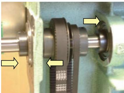
(3) Position of upper pulley is [2mm] from upper shaft collar.
