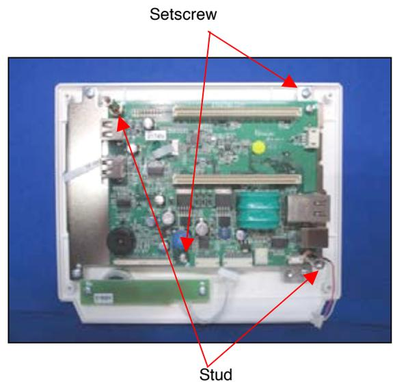
7. Lift LCD-CE board as shown in the figure below.
