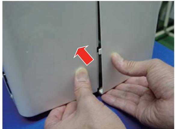
15. Remove the cover by pressing an arrow part of the picture.
