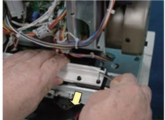
5. Assemble detecting plate.
