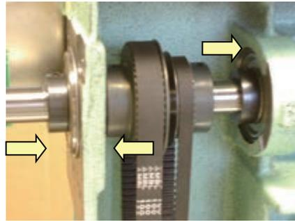
(3)Position of upper pulley is space from upper shaft collar.
