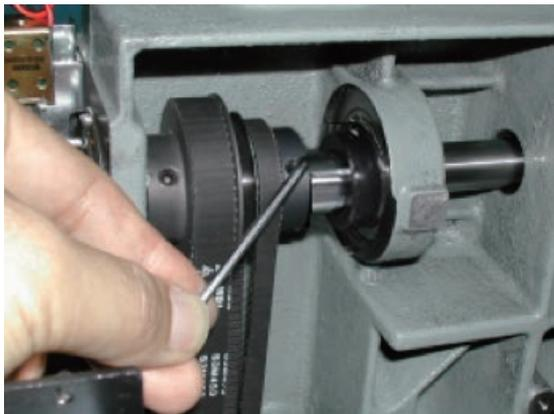
11. Loosen collar screw on take-up lever cam.
