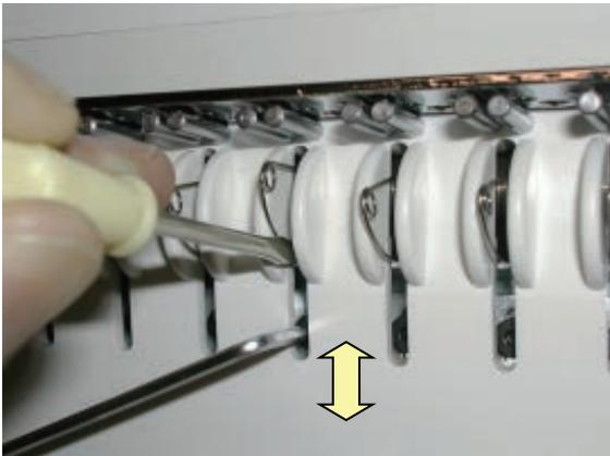
3. After adjustment, tighten screw to finish.
