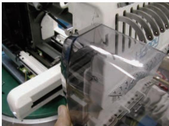
4. Remove thread tension bracket.
