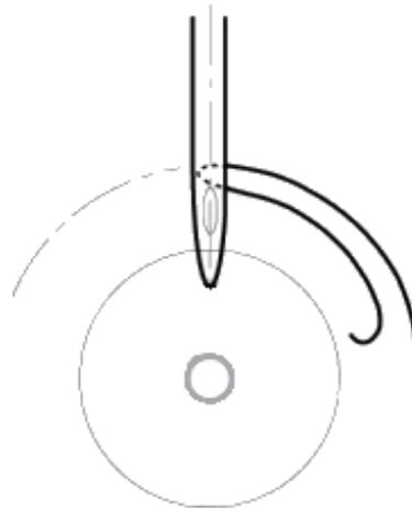
At this moment, clearance between needle and rotary hook should be [0.1-0.2mm].
