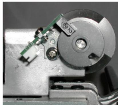
3. After installation, please fix potentiometer referring to [3-4-2 Setting to detect needle position].
