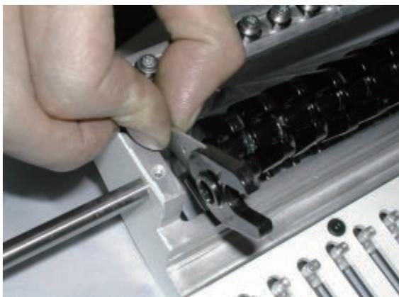
9. Install good take-up lever assembly with plastic washer, E-ring.
