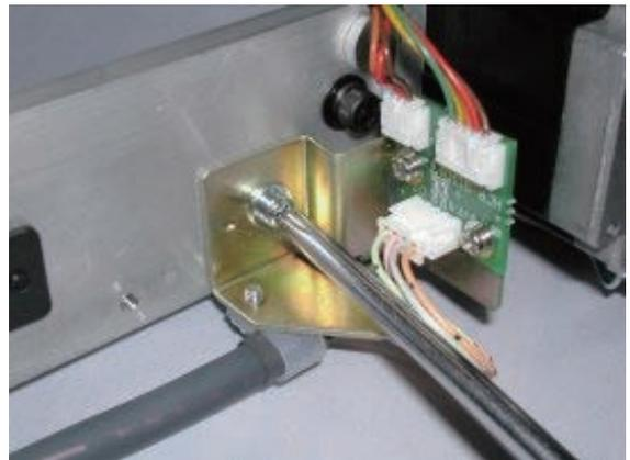
6. Loosen fixing screw for tension pulley bracket slightly.
