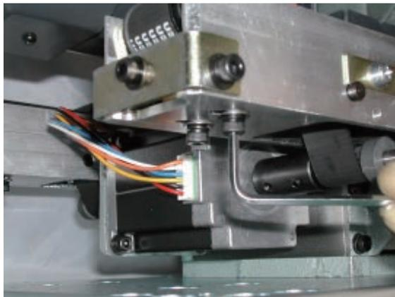
7. Loosen screw for tension.
