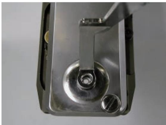
6. Insert thickness gauge [1.2mm] between needle plate and pressure foot then tighten the screw which fixes guide bar block.
