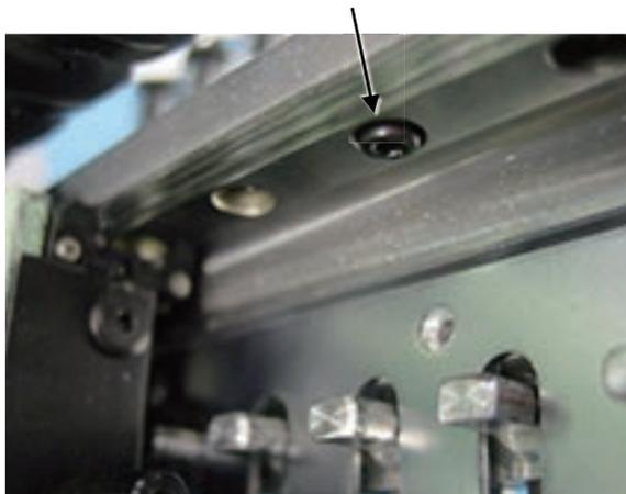
3. Put in SIMM [0.05mm] between a moving head and LM guide.
