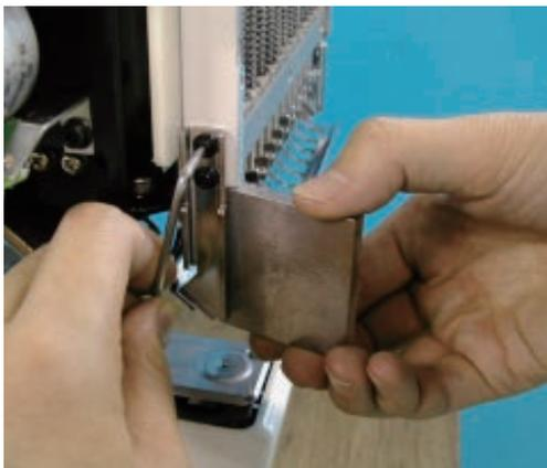
4. Hold down the pressurefoot and take the hook in and out by finger to check movement of hook goes smoothly.
