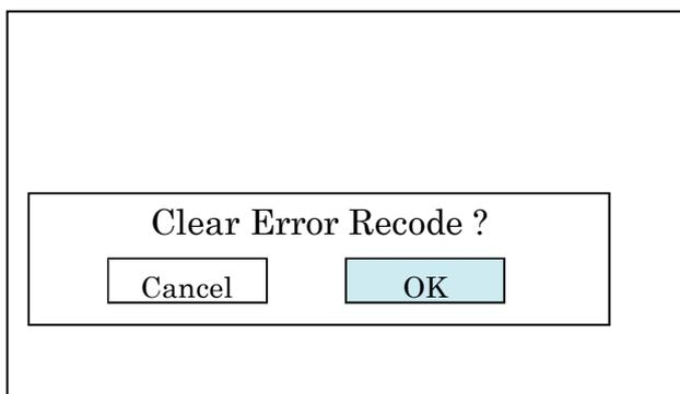
\* Error record is cleared by pressing **OK** and the screen of the procedure 3 is displayed.
