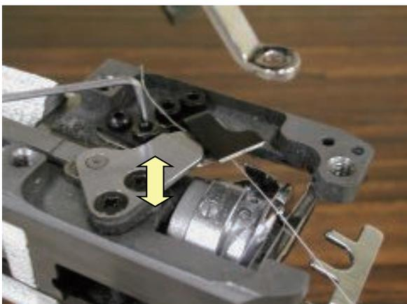
4. Pull bobbin thread toward arrow mark and see that bobbin thread comes off with tensile gauge [20-25g].
