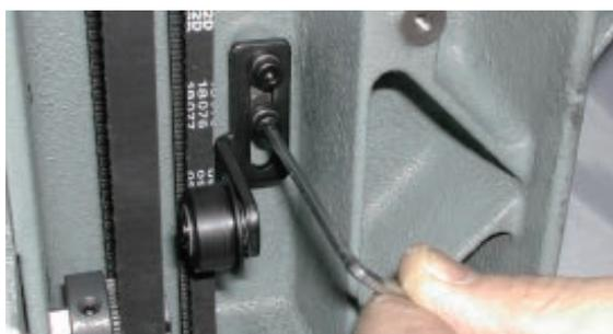
3. Loosen screws on upper shaft collar,
