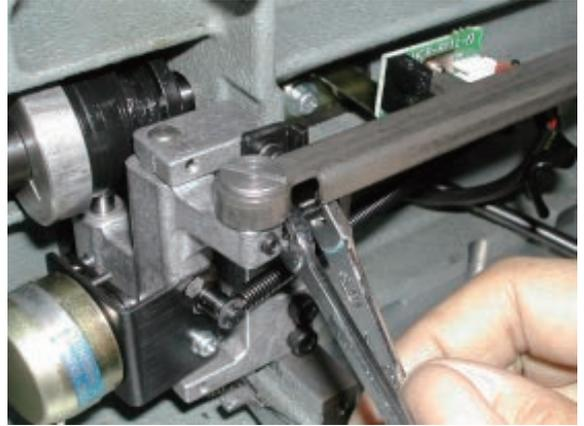
6. On checking the clearance [0.2mm] between cam and roller by using 0.2mm thickness gauge.
