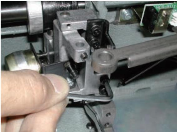
12. Fix drive link ass'y to thread cutting driver ass'y.
