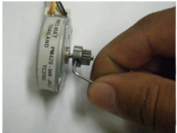
9. Install Drive gear on good Pulse motor
