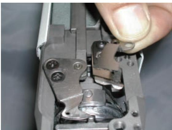
4. Tighten fixed knife pushing to forward as full as possible.
