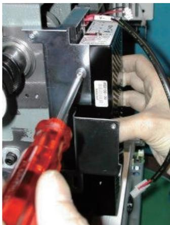
2. Remove timing detecting board ass'y.
