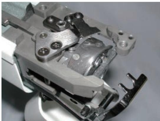
6. With release lever being pushed down, turn upper shaft to open and close moving knife repeatedly.
