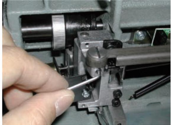
8. Remove thread cutting driver ass'y .
