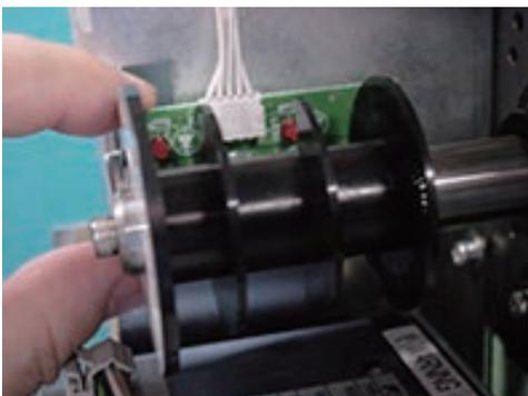
5. With this state, turn to C point and check if LED1 lights between [265 and 282 degrees].
