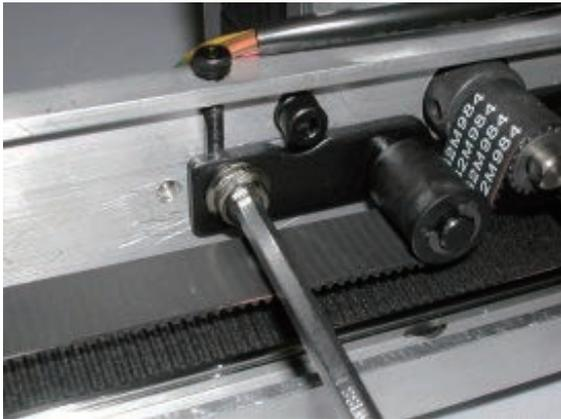
8. Loosen screw (rear) slightly to the extent that tension-bracket moves.
