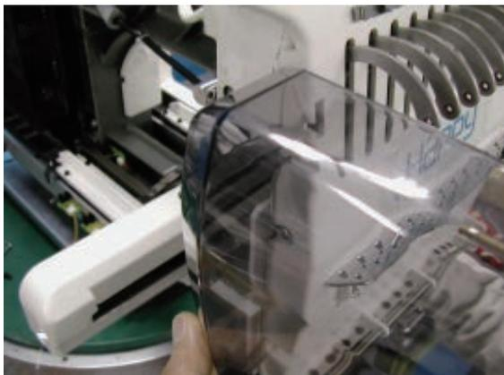
4. Remove thread tension bracket.
