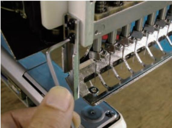
3. Insert positioning gauge [ $47.5 \pm 0.1 \text{mm}$ ] between lower part of moving head and holder (upper) and mount it vertical.
