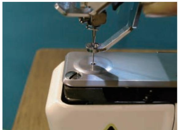
4. After adjustment, please be sure to check and adjust clearance between needle and shuttle hook.
