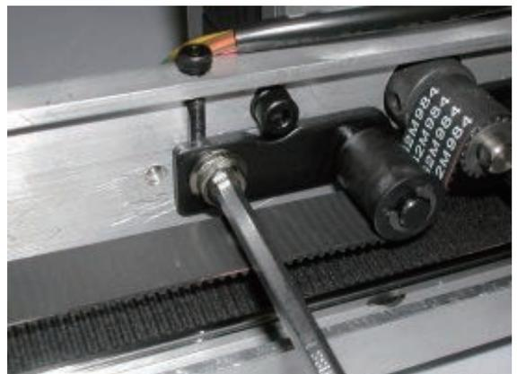
7. Loosen fixing screw for tension pulley bracket slightly.
