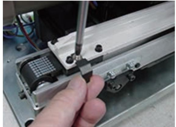
6. Check of interference between detecting plate and sensor or connector of sensor board.
