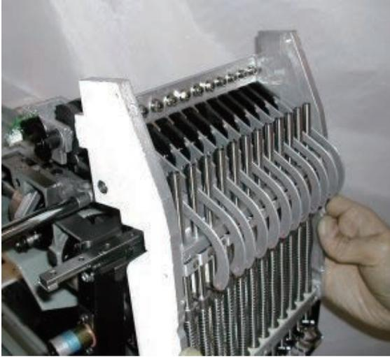
2. Exchange of needle bar boss guide plate.
