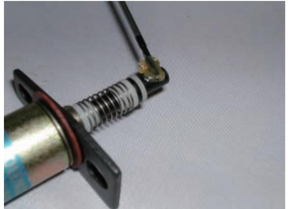
4. Assemble the solenoid to the original position.
