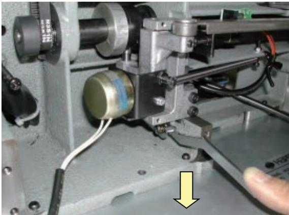
4. Insert 0.2mm thickness gauge between cam and roller and adjust the clearance [0.2mm] between cam and roller by adjusting screw.)
