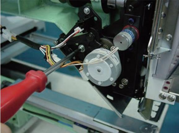
2. Tighten thread catcher pushing it upward and forward.
