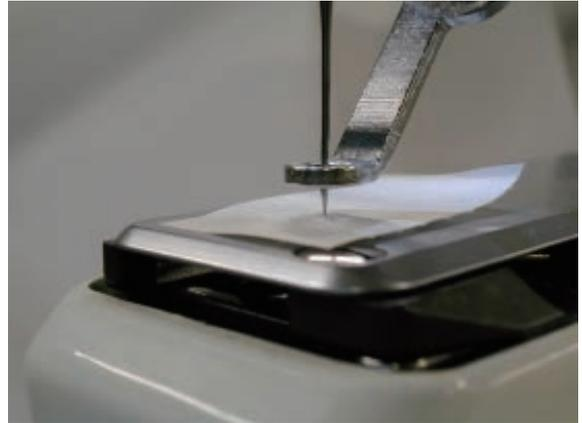
7. Reverse-rotate an upper axis, raise a needle bar, and unite with C [275 degrees].
