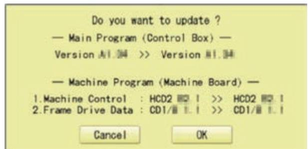
9. When the current machine program is older than latest version, press **OK**.
