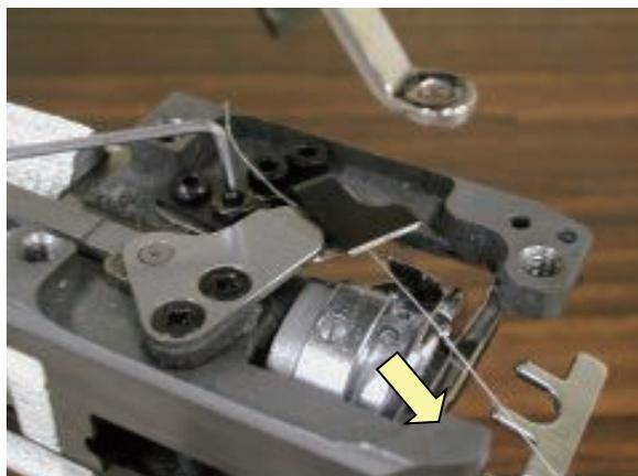
5. Tighten lock nut. (Don't move adjusting screw.)
