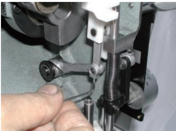
4. If you remove the pressure foot link B ass'y, first remove the pressure foot cam collar and pressure foot drive cam.
