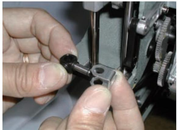
6. Assemble the pressure foot guide bar and pressure foot.
