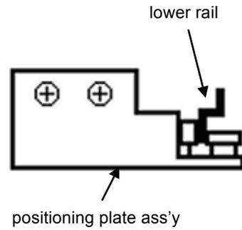
Viewing from side, set to center of needle hole.
