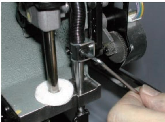
3. Rotate the upper shaft to be lowest point [0 degrees].
