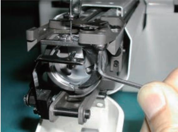
2. Install screw for Needle plate. (only front side)
