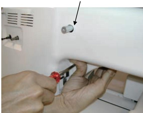
3. Assemble thread tension ass'y.
