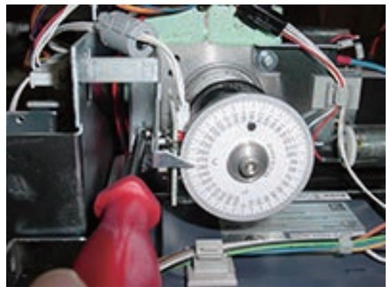
9. Remove bobbin winder and power supply.
