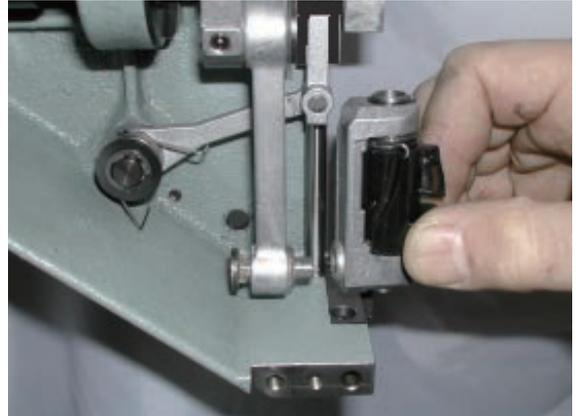
8. Remove circuit board assembly for timing detecting board.
