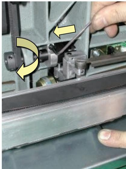
5. Tighten screw on thread cut cam when moving knife began to open.
