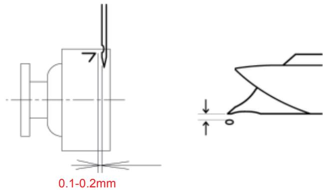
7. For making sure, check position of retainer on bobbin case holder.
