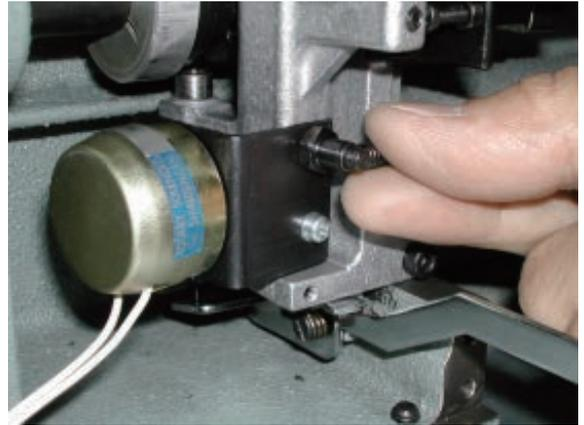
14. Fix Y carriage bracket (left) to the machine.
