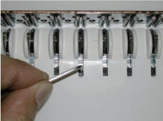
2. Move adjuster position up and down with small flat-head driver to change stroke.
