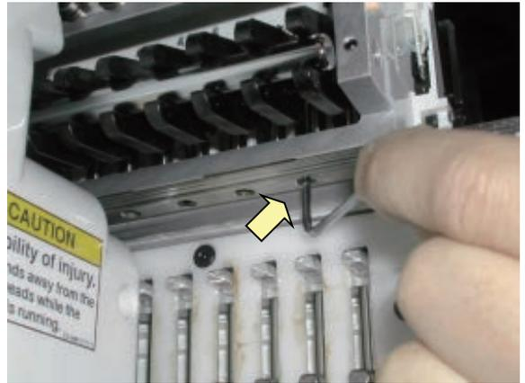
8. Turn the drive shaft B screw for manual operation, and make it the 12th needles.
