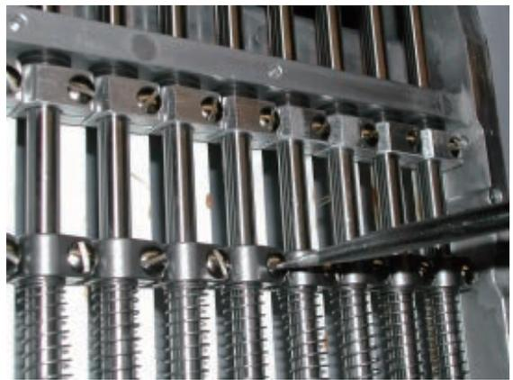
11. Tighten the screw of needle bar boss B.
