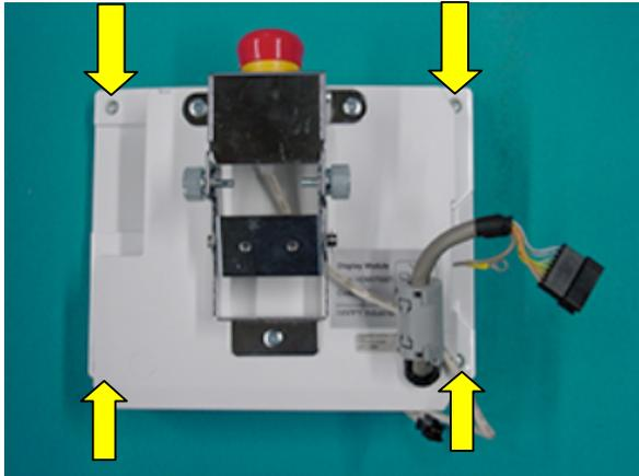
2. Remove connectors for SW cable, Box cable, cable for LCD inverter (red/white).
