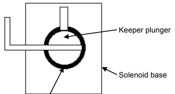
Clearance between keeper plunger and solenoid base should be kept as much as equally.
