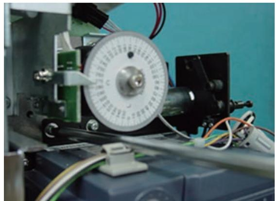
6. Adjust bobbin thread tension [30g] by tension gauge.
