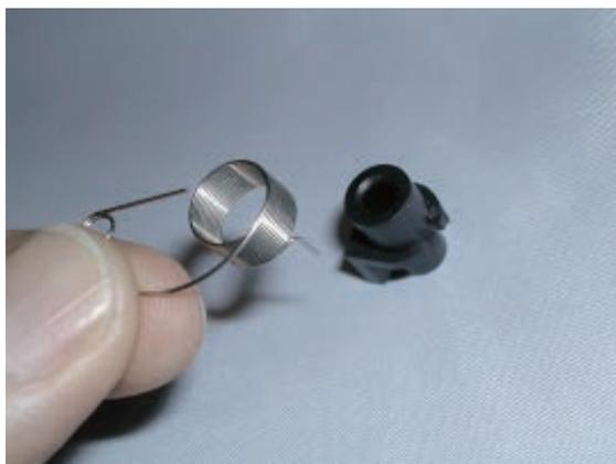
6. Assemble the thread adjusting spring into lower front panel.
