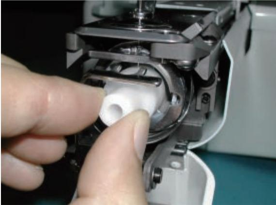
8. Adjust the needle bar height up and down till the needle tip touches to the gauge slightly.
