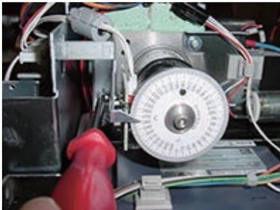
3. Loosen screws on upper shaft collar, upper pulley and drive pulley.
