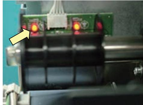
\* Check dose not scratch plastic slit to Timing sensor.
