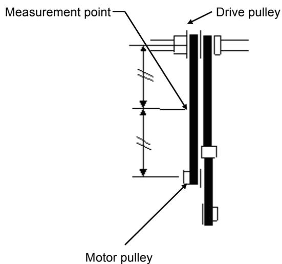
Adjust of tension should be 320 – 330g at belt is pressed 3mm.
