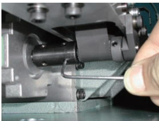
4. Remove the screw of Y carriage bracket (left).
