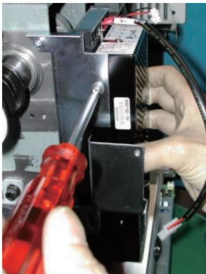
2. Remove timing detecting board ass'y.
