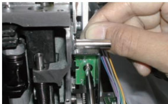
5. Exchange pressure foot drive lever ass'y.
