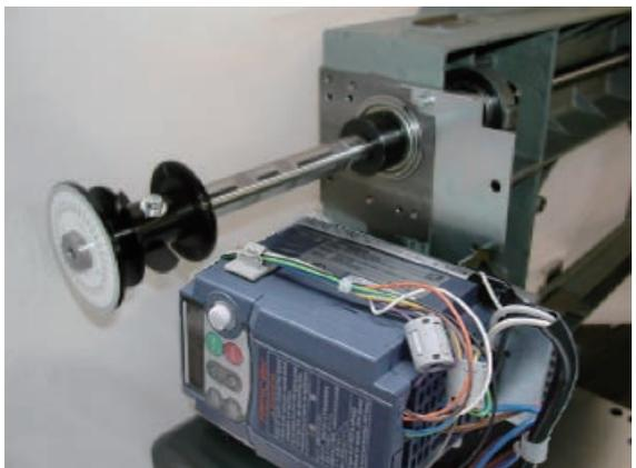
7. Remove drive pulley and motor belt.
