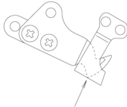
Adjustment of clearance between moving knife and fixed knife is where both tip of them are attached.
