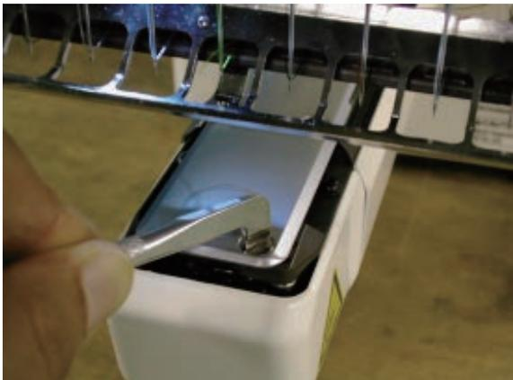
2. Check if knife drive shaft has no backlash in up and down direction.
