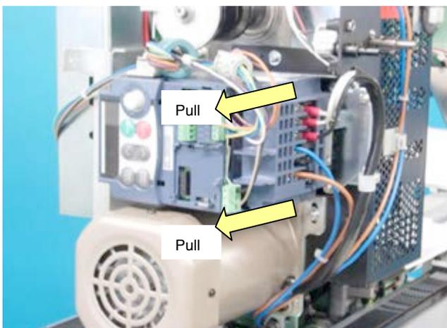
4. Loosen screw with Phillips screwdriver for precision instrument and remove 9 cables. (Cable color: ORANGE, BROWN, PURPLE, WHITE, GREEN, BLUE, YELLOW, BLACK, and GLAY)
